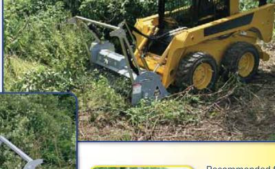
Recommended for: high performance brush cutting on highflow hydraulics of up to 40<sub>GPM</sub>. The MF760 is a perfect fit for the midsize or largest skid steers available.
